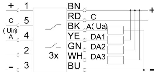
DA1/DA2/DA3 Digital switching outputs ( closing )
