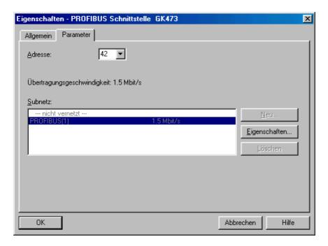
In this window enter only the Node ID which has to be identical to that previously set at the gateway's two rotary switches (Example: 42).
