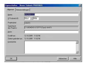
Next step is connecting the gateway to Profibus. HW Config → Catalogue → other fieldbus devices → Gateway → GK473. Drag name "GK473" to the dotted Bus rail using the left mouse key.
