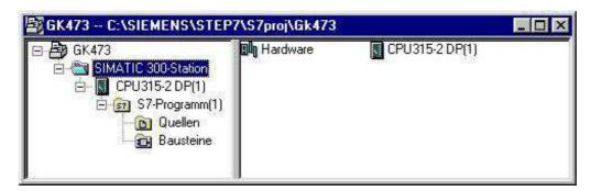
The hardware window of the Simatic Manager as independent program element "HW config" will open.
