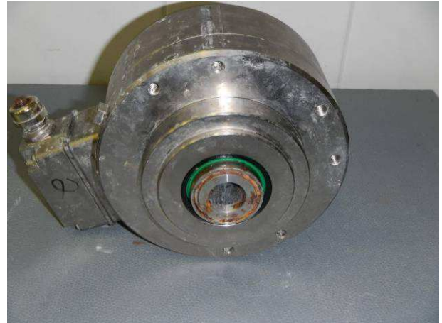
Picture 14 Incremental encoder HOG165C DN 1024 I with red rust on the bearing after the salt mist Kb
