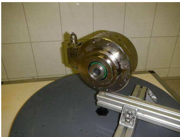
Picture 5 Incremental encoder HOG165C DN 1024 I without any alterations after the protection against water jets test IPX6
