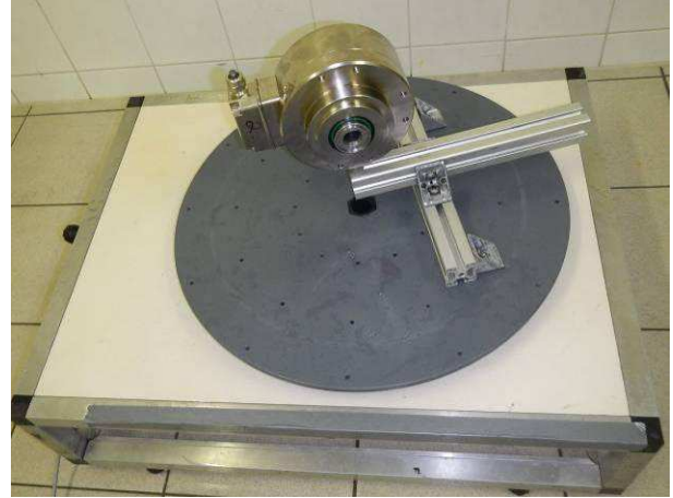
Picture 2 Incremental encoder HOG165C DN 1024 I mounted on the turn table before the protection against water jets test IPX6
