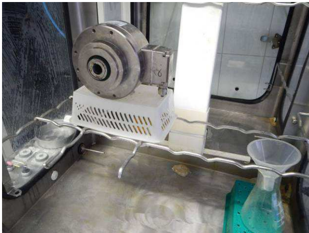
Picture 9 Incremental encoder HOG165C DN 1024 I in the salt mist chamber 47 before the salt mist Kb
