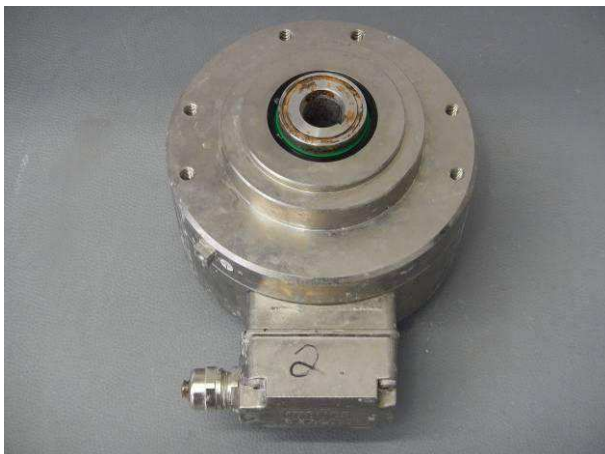
Picture 11 Incremental encoder HOG165C DN 1024 I with visible corrosive alterations after the salt mist Kb
