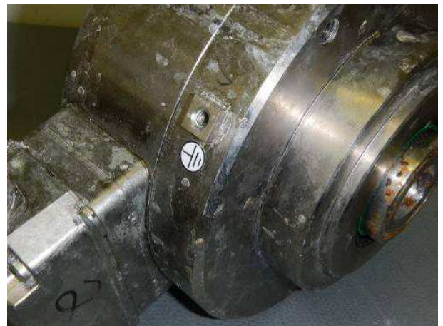
Picture 16 Incremental encoder HOG165C DN 1024 I with visible corrosive alterations after the salt mist Kb
