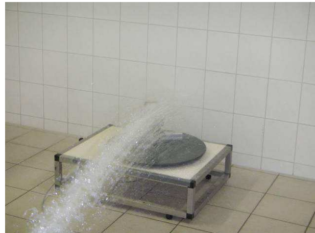
Picture 4 Incremental encoder HOG165C DN 1024 I on the turn table with standardized water jet during the protection against water jets test IPX6
