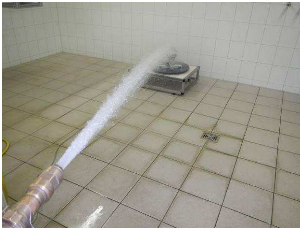
Picture 3 Incremental encoder HOG165C DN 1024 I on the turn table with standardized water jet during the protection against water jets test IPX6
