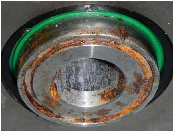
Picture 15 Incremental encoder HOG165C DN 1024 I with red rust on the bearing after the salt mist Kb
