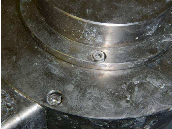
Picture 13 Incremental encoder HOG165C DN 1024 I with dark spots and white deposits after the salt mist Kb
