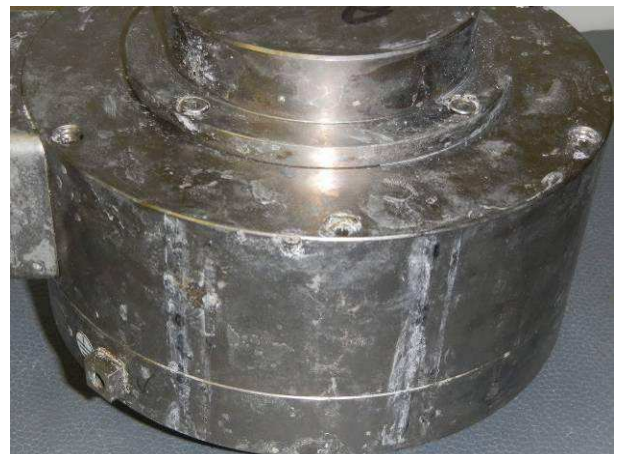
Picture 12 Incremental encoder HOG165C DN 1024 I with dark spots and white deposits after the salt mist Kb
