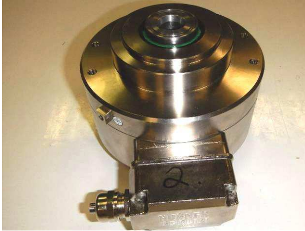
Picture 1 Incremental encoder HOG165C DN 1024 I delivery status before the protection against water jets test IPX6
