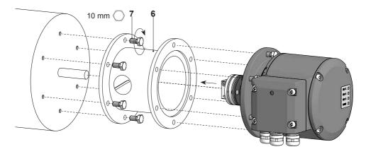
The encoder must be mounted with cable connection facing downward and not exposed to water.
