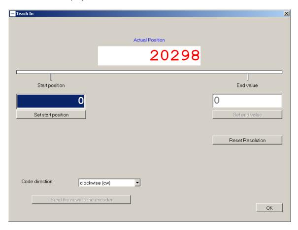
In the field "current position", the current value of the encoder with max. resolution is displayed.
