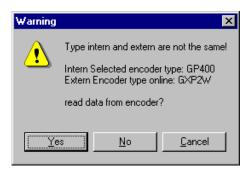
If the selected type of encoder and the connected one are identical, the data will be read in and displayed.
