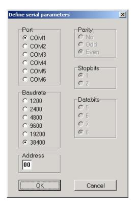
Click "settings" menu to select the serial interface COM 1 up to COM 6 to which the encoder is connected. Furthermore, you can adjust the baud rate and the address of the encoder. The other parameters such as parity, stop bits and data bits can be controlled here.
