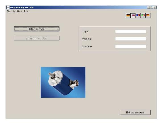
The programming can only be started after selecting a type of encoder. The selection of the encoders is described in the chapters "Encoder connected to  $PC \Rightarrow$  Automatic selection" and "Select type of encoder from table  $\Rightarrow$  Manual selection".
