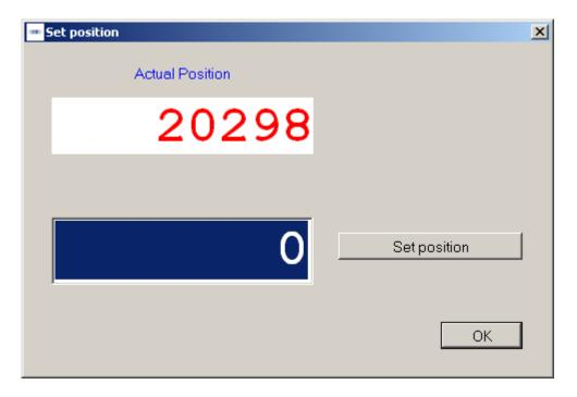
To the encoder models GXP1H, GXP1W, GXP2W with version 2C applies the following: After having assigned the preset value by the "set position" function, the external reset input must not be used.
