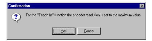
Click "Yes" to confirm the setting of the encoder to the maximum resolution. The following window will be displayed:
