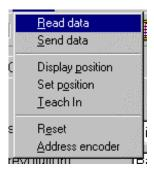
Call up data: The data is called up from the connected encoder Send data: The current programming is saved in the encoder
