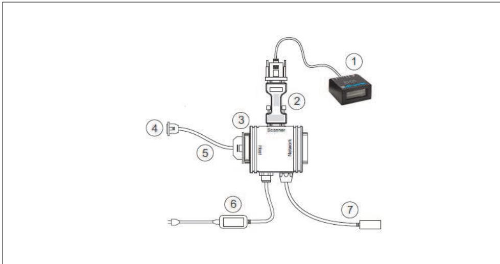
Figure 1-2 ID-01 Hardware Configuration
