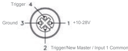
Trigger Connector 4-pin Socket
