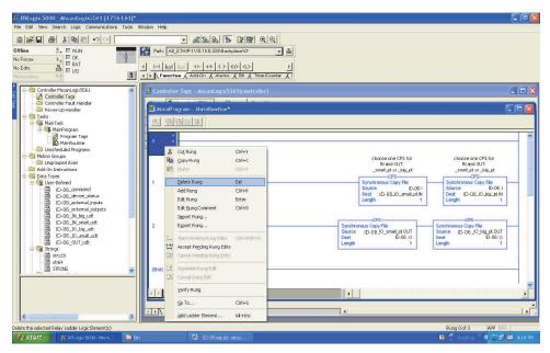
15. Select one CPS instruction per rung, the "\_small\_pt" on the left, or the "\_big\_pt" on the right. Keep the one that corresponds to the assembly sizes configured for the module, and delete the other:
