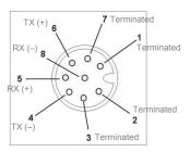
B (Ethernet Models) M12 8-pin Socket
