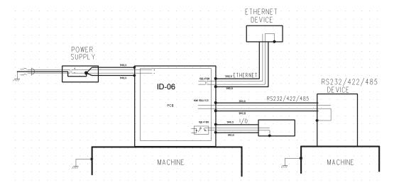
An earth ground is provided through the cable shields and chassis of the imager.
