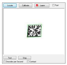
The symbol in the field of view will appear in the video view beneath the **Locate** and **Calibrate** buttons, and you will see the red target pattern projected from the front of the imager.
