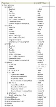
RS-232 A, RS-232 B, and RS-422 are serial. RS-232 A is always enabled. RS-232 B and RS-422 can be enabled or disabled to match the physical requirements of the application. Ethernet can also be enabled or disabled as required.
