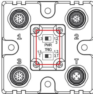
**Power** can be bussed between imagers and interface devices. At each location on a network where a new power supply is added, the Power switch on the VSID-IB-ES can be used to break power between Connector 2 and Connectors 1, 3, and T.
