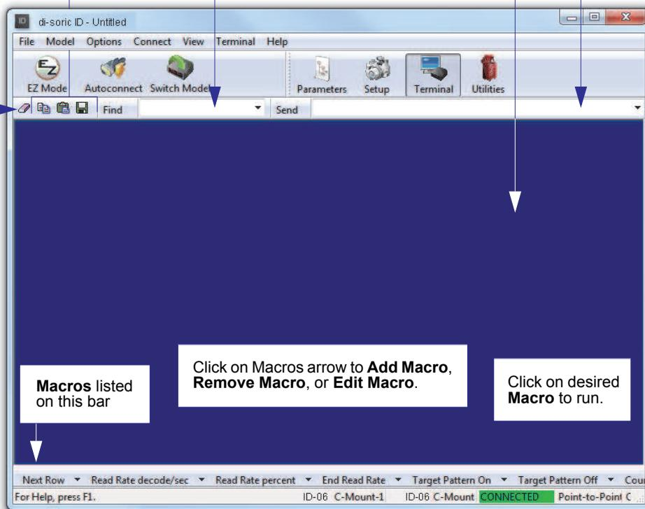
The **Terminal** interface allows the user to send serial commands to the imager by using macros, by copying and pasting, or by typing commands in the **Send** text field.
