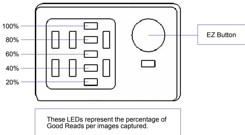
2. To end the Read Rate test, press the EZ Button and quickly release.
