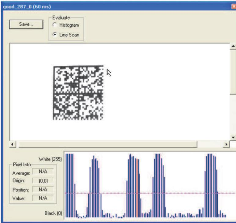
When you center your cursor over the dashed line, it becomes a double arrow cross. This allows you to move the line anywhere in the window. You can also use your keyboard arrows to move the line incrementally in any direction.
