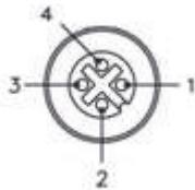
**VSID-IB-ES Trigger Connector 4-pin**
