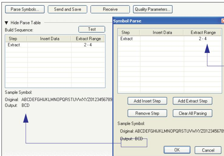
Multiple character sequences can be extracted and inserted using **Symbol Parse**. In this example, the selected extraction range is characters 2-4. The "Sample Symbol" example on the **Symbol Parse** dialog shows the selected character positions extracted and output as desired. Simultaneously, the data string from the selected symbol is displayed at the bottom left of the **Parse Table**, followed by the user-defined extracted output.
