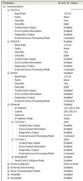
**RS-232 A, RS-232 B, and RS-422** are serial. RS-232 A is always enabled. RS-232 B and RS-422 can be enabled or disabled to match the physical requirements of the application. **Ethernet** can also be enabled or disabled as required.
