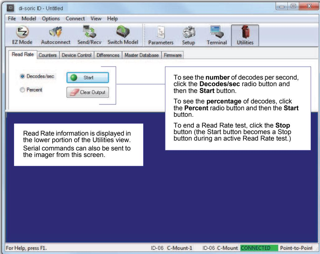
Read Rate information is displayed in the lower portion of the Utilities view. Serial commands can also be sent to the imager from this screen.
