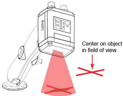
**Important:** The entire symbol should fall within the field of view (FOV) of the imager. The field of view is what appears in **di-soric ID's Locate/Calibrate** window in **EZ Mode**.
