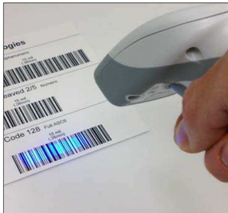
As you draw the reader away from the symbol, the two bars converge. At the optimal distance, the two bars should just be touching, as shown above.
