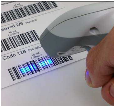
When the reader is closer to the symbol, you will see two separate bars.
