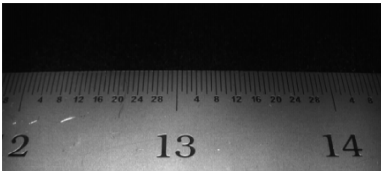
FIGURE 3–2. Off-Axis – Semi-Specular Surface (Fine Matte Metal Ruler) at 2", 90°
