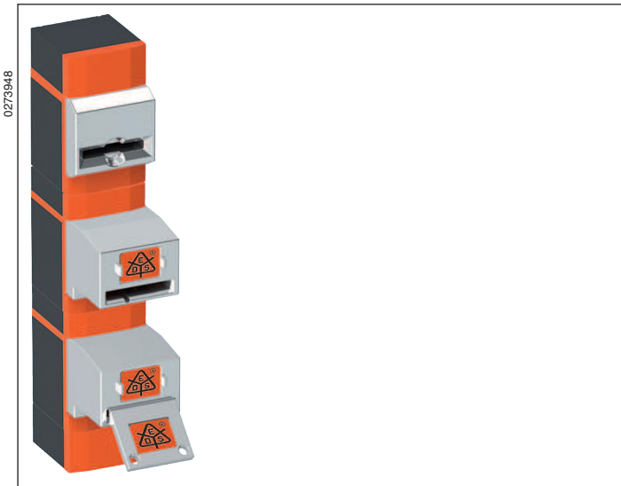
Presentation in the deactivated condition: 1st key inserted; 2nd key and actuator removed
