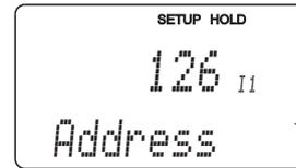
**Setting the device address via PROFIBUS communication**
