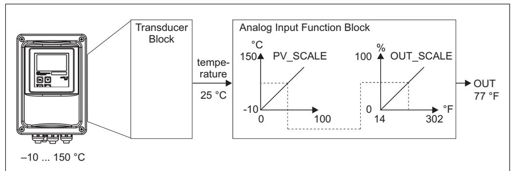
Fig. 11: Scaling the input value for the Analog Input function block
