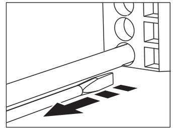
Fig. 6: Remove the screwdriver (closes the terminal)
