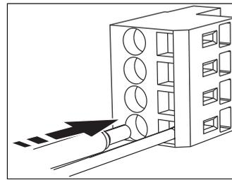
Fig. 5: Insert the cable until the limit stop
