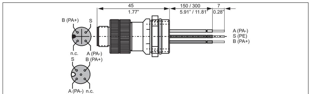
Fig. 16: M-12 plug with socket
