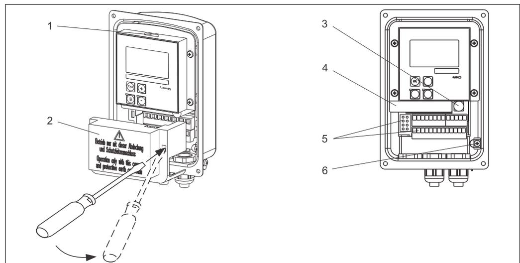
Fig. 2: Bus cable connection Smartec S PROFIBUS
