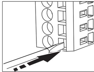
Fig. 4: Insert the screwdriver (opens the terminal)
