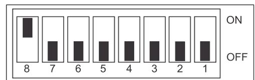
Fig. 13: Factory setting of the DIL switch
