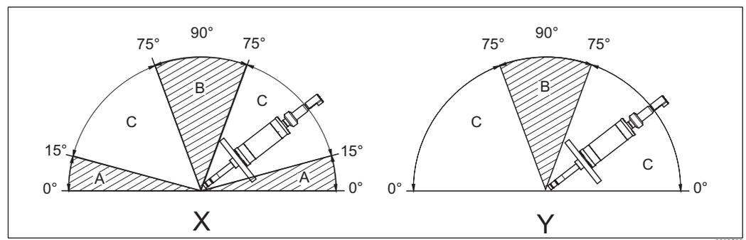
Fig. 1: Installation angles for glass sensors (X) and ISFET sensors (Y)
