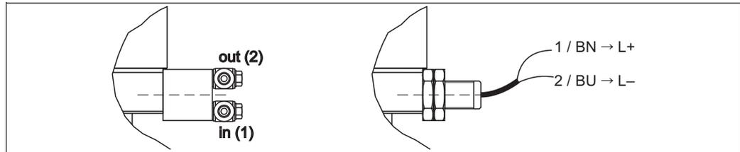
Fig. 9: Limit position switches, left: pneumatic (1 = compressed air inlet, 2 = compressed air outlet)
