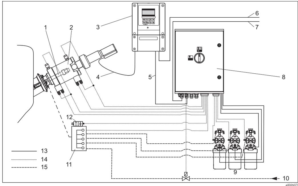
Fig. 7: Measuring system with pneumatic control
