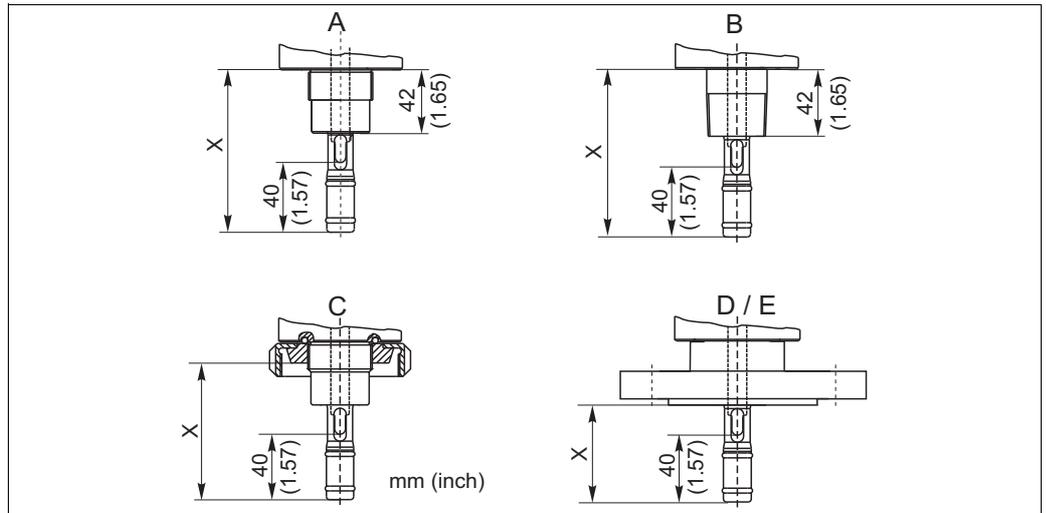
Fig. 6: Process connections short version / long version
