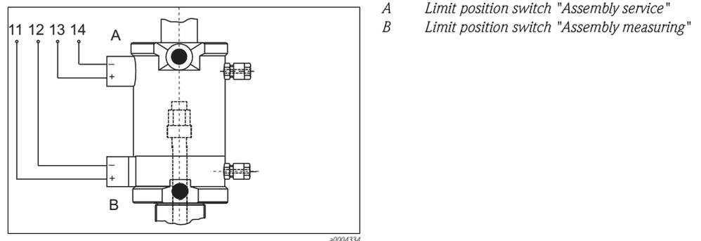
Fig. 11: Electric limit position switches to Topcal
