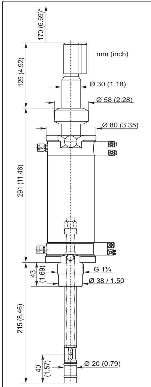
Fig. 3: Long version for gel sensors
