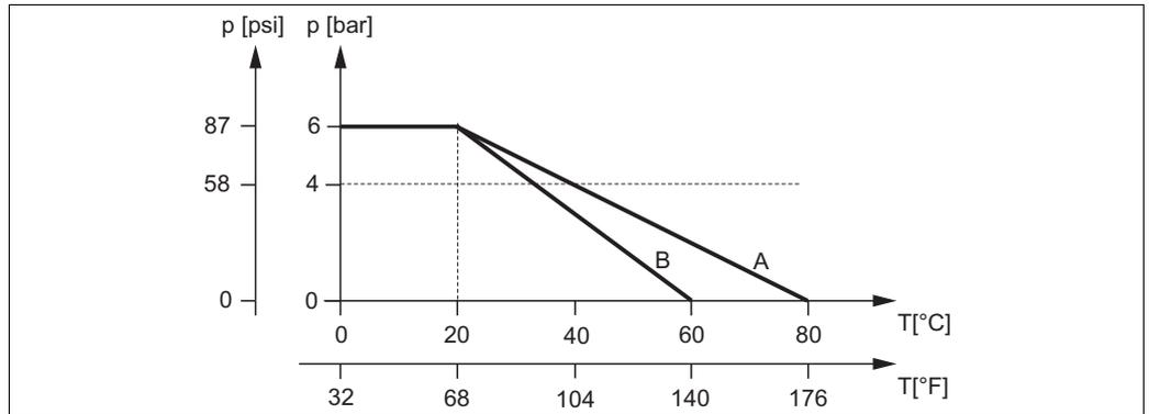
Fig. 25: Pressure temperature diagram
