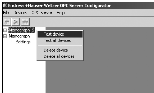
Fig. 5: Testing the connection
