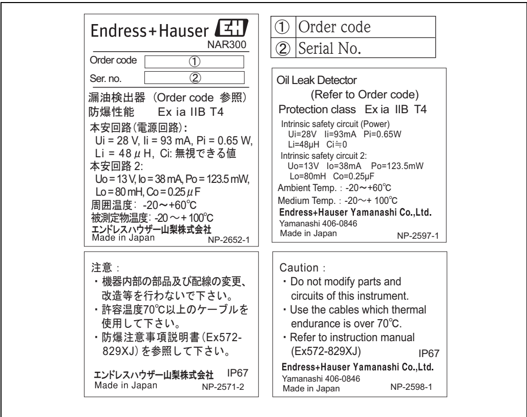
Figure. 2: High Temperature Type (NAR300-16xxxx)
