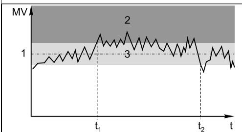
The hysteresis is needed to ensure a stable switching behavior.
