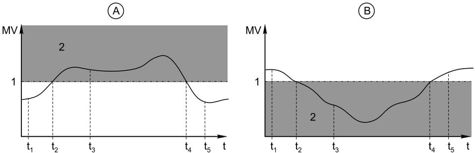
Fig. 12: Exceeding (A) and undershooting (B) a limit value (without hysteresis and switch-on delay)
