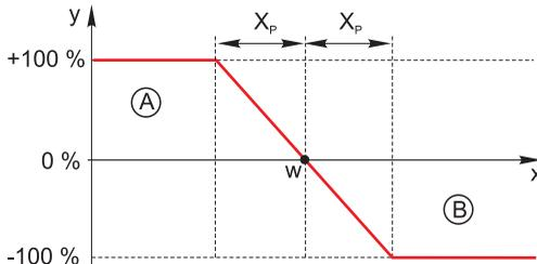
The red curve shows overlap between the curves of the two 1-sided controllers.
