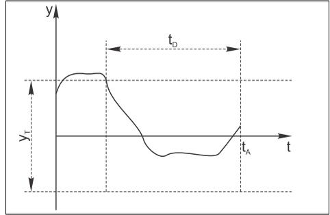
Fig. 8: Stagnating signal, alarm is triggered
