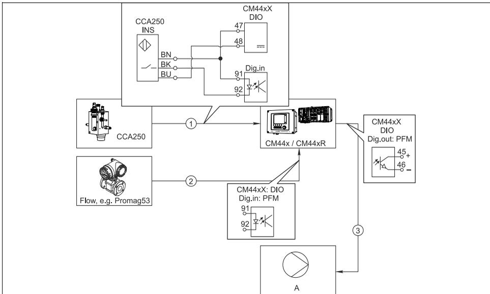
Fig. 10: Example of chlorine control with feedforward control
