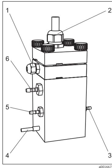
Fig. 3: Collecting vessel
