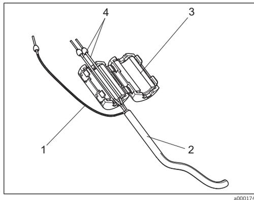
Fig. 14: Interference protection of the signal cable
