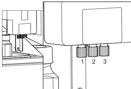
2. Mount the Pg M25 gland supplied on the device floor from the outside.
