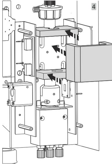
5. Put the cover back on the reactor and fix it in place with the screws.
