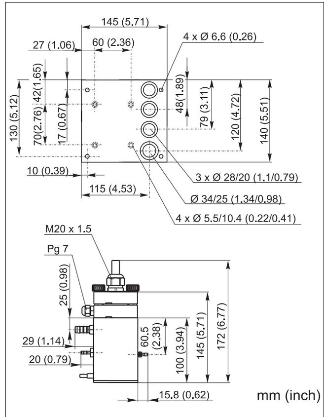
Fig. 4: Dimensions of collecting vessel and base plate
