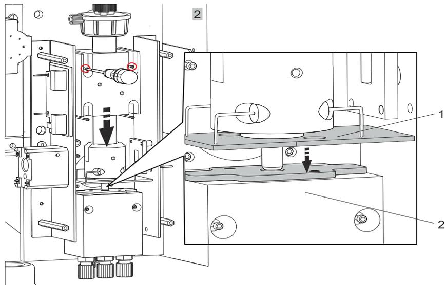
3. Fix the cooling block in place with the screws.
