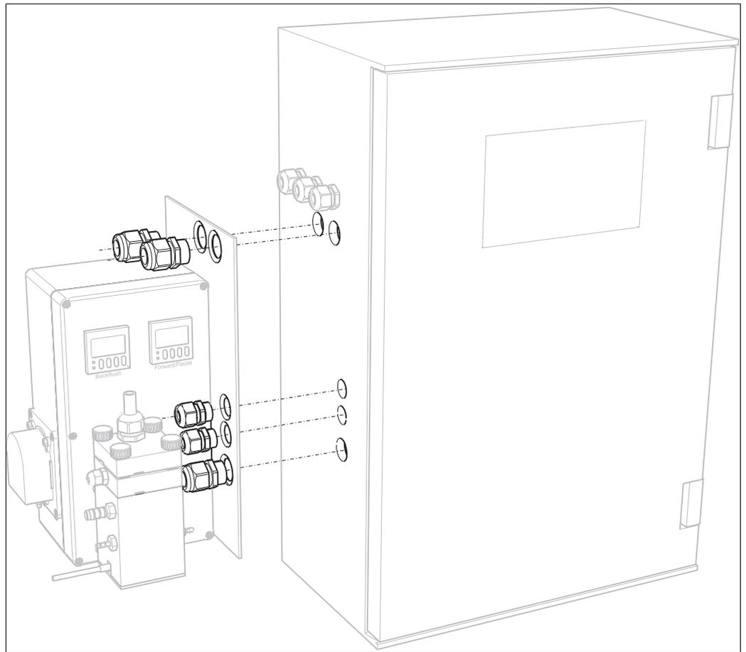
Fig. 8: Installation of the back-flush pump unit
