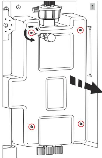
2. Release the screws of the cooling block and **carefully** move the entire reactor downwards until the printed circuit board (1) rests flush on the valve manifold (2).
