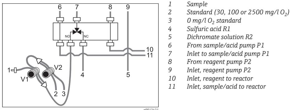
Fig. 7: Valves and valve hoses
