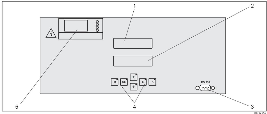
Fig. 15: Display and operating elements
