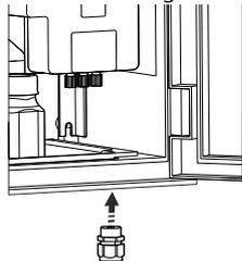
3. Route the drain hoses (PTFE 4/6 mm) through the gland boreholes to the outside.
