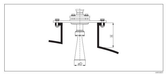
$\blacksquare$  8 Nozzle height and diameter for the horn antenna (FMR57)
