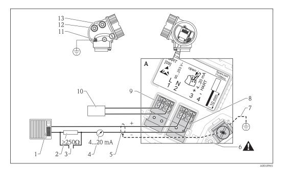
■ 16 Terminal assignment 4-wire; 4-20mA HART (90 to 253 VAC)
