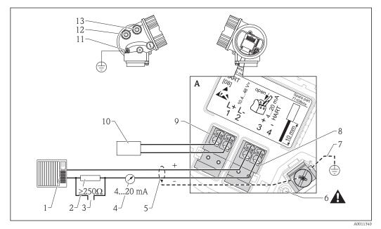
■ 15 Terminal assignment 4-wire; 4-20mA HART (10.4 to 48 VDC)
