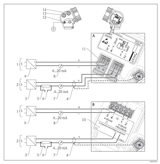
图 14 🛮 Terminal assignment 2-wire, 4-20 mA HART, 4...20mA
