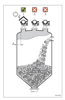
Recommended distance A from wall to outer edge of nozzle: ~ 1/6 of vessel diameter.
