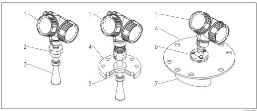
**₽** 2 Design of the Micropilot FMR57 (26 GHz)
