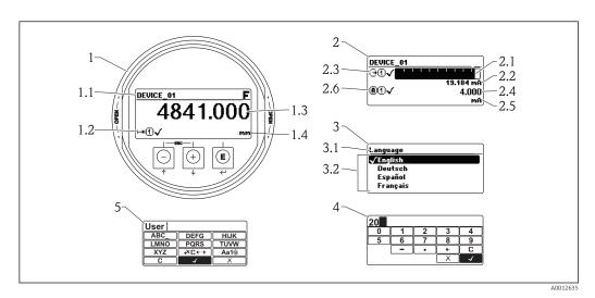
$\blacksquare$  21 Appearance of the display and operation module for on-site operation
