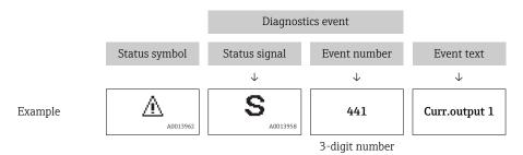
If two or more diagnostic messages are pending simultaneously, only the message with the highest priority is shown. Additional pending diagnostic messages can be shown in the **Diagnostics list** submenu ( $\rightarrow \implies 134$ ).
