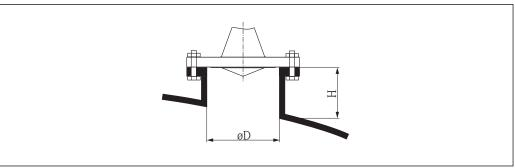
€ 6 Nozzle height and diameter for horn antenna with slip-on flange (FMR50/FMR56)
