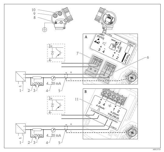
■ 13 Terminal assignment 2-wire; 4-20mA HART, switch output
