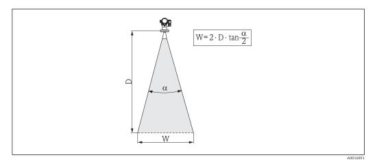
$\blacksquare$  5 Relationship between beam angle  $\alpha$ , distance D and beamwidth diameter W
