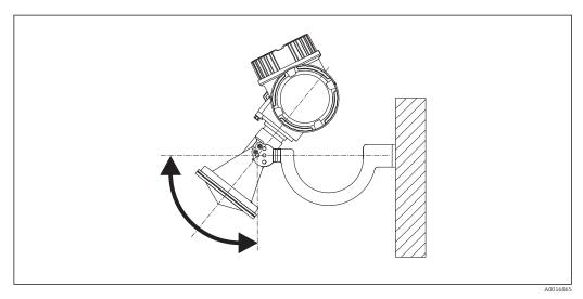
$\blacksquare$  7 Installation of the horn antenna with mounting bracket (FMR50/FMR56)
