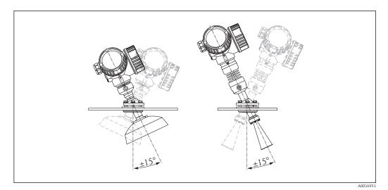
$\blacksquare$  10 Micropilot FMR57 with alignment device
