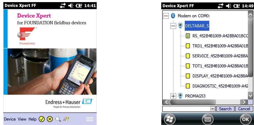
Fig. 2-1: Device Xpert FOUNDATION fieldbus start page and live list of connected devices
