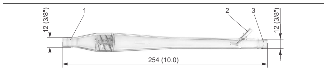
Fig. 37: Bubble trap, dimensions in mm (inch)
