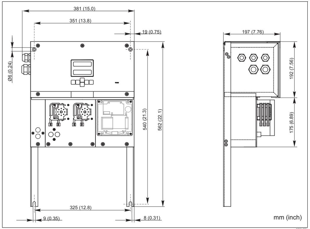
Fig. 5: Version without housing (open design)
