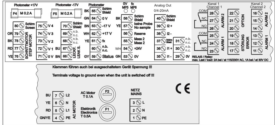
Fig. 16: Example of connection stick-on label
