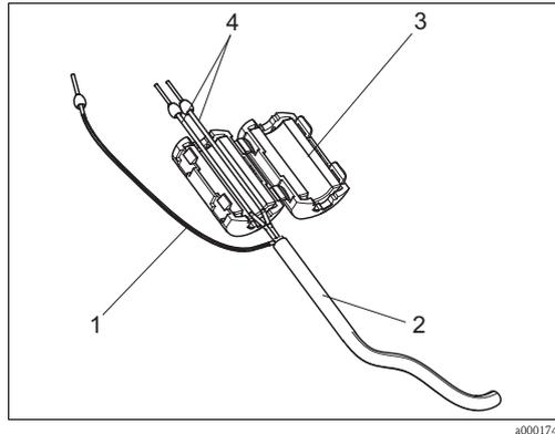
Fig. 18: Interference protection of the signal cable
