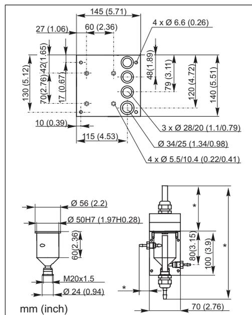
Fig. 7: Dimensions of collecting vessel and base plate
