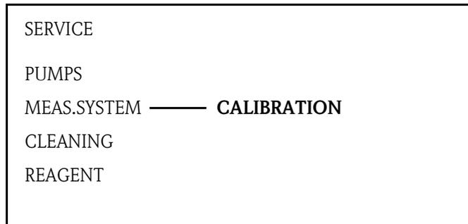
Fig. 40: MEAS.SYSTEM/CALIBRATION service menu
