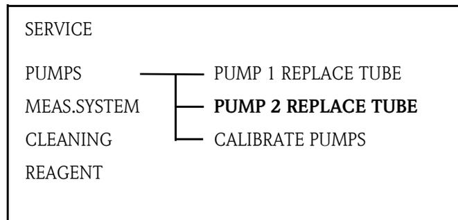
Abb. 27: PUMP 2 REPLACE TUBE service menu
