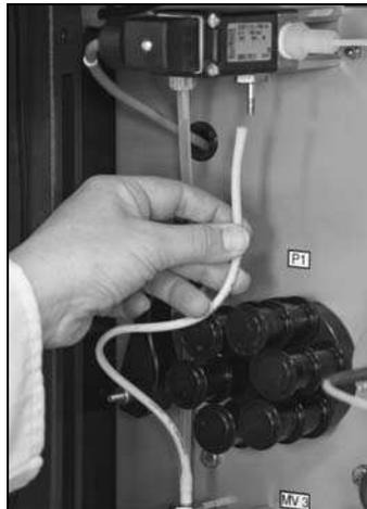
Fig. 24: Releasing the tube connection nipples
