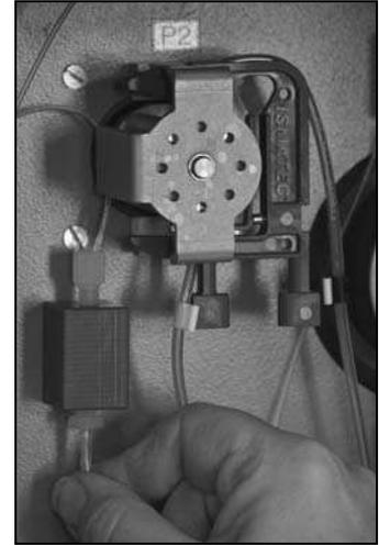
Fig. 30: Tube connection to connection block, pump P2
