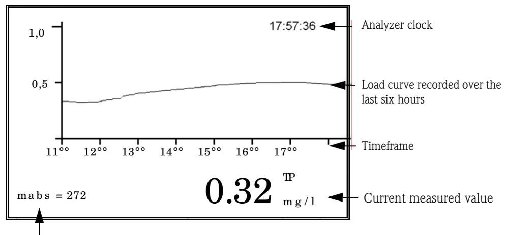
mabs: = indicates the current absorption in the measuring cell (mabs: milliabsorption)
