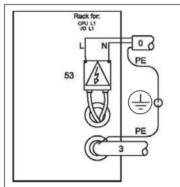
Fig. 6: Sample wiring diagram for connection to mains
