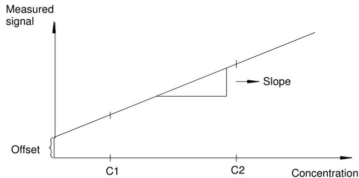
Fig. 38: Analyzer calibration line
