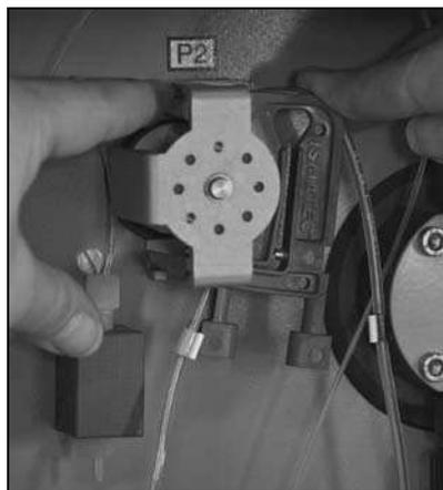
Fig. 31: Removing the tube case, P2
