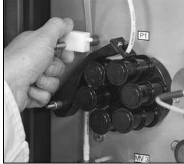
Fig. 22: Opening the tube bed throttle
