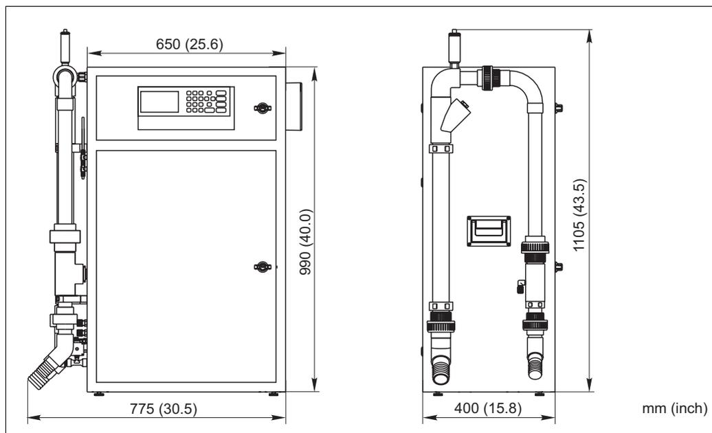
Fig. 4: Dimensions including sample conditioning PA-2 (option)
