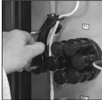
Fig. 23: Opening the tube bed
