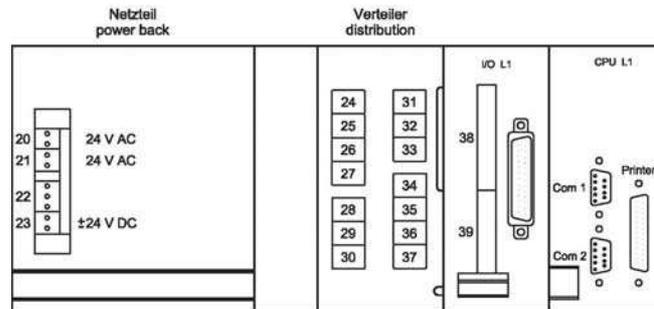
Fig. 9: Example of electronics frame wiring diagram
