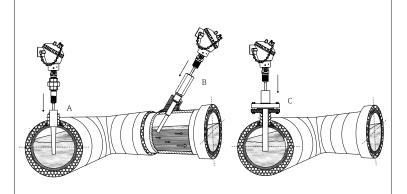
Examples of spring loaded insert installation:
