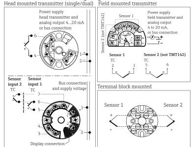
Wire specifications: Thermocouple grade, TFE insulated 20AWG, 7 strands with stripped ends
