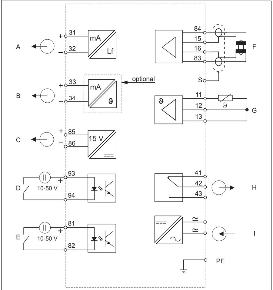
Fig. 3: Electrical connection of Smartec S CLD134
