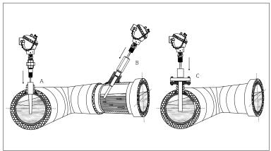
Examples of spring loaded insert installation.
