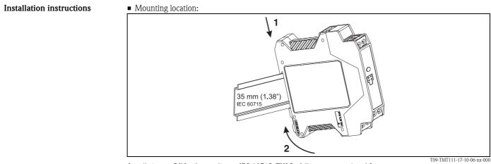
Installation on DIN rail according to IEC 60715, TH35 - follow sequence 1 and 2
