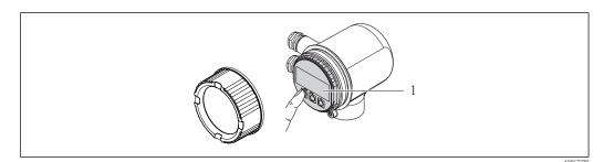
1 Display module (pushbutton operation)
