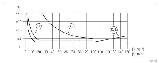
**5** Maximum measured error (% mass flow) as % of measured value/full scale value. G, H, K, L: Order code options for "Calibration flow", see the following table
