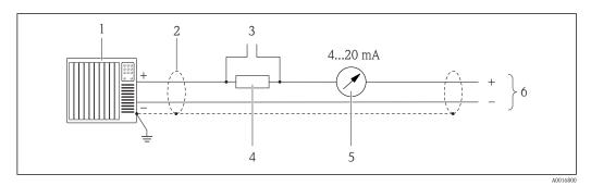
2 Connection example for current output, 4-20 mA HART active
