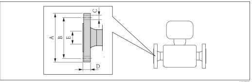
Fixed flanges as per ASME B16.5 / Cl 300 A [in] DN С D Е [in] [in] [in] [in] [in] 1/2 3.74 2.63  $4 \times Ø5/8$ 0.91 0.62 3.5  $4 \times Ø3/4$ 1.06 1.1 1 4.92
