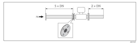
6 Recommended inlet and outlet runs when using a flow conditioner
