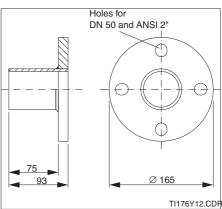
right: Welding socket for pipe diameter greater than 80 mm
