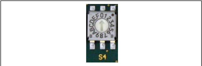
Figure 8.5: Rotary switch for device selection
