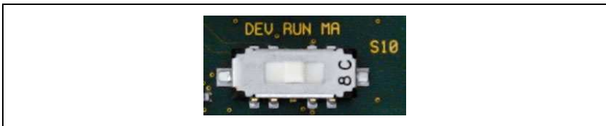
Figure 4.2: Service-switch switch positions
