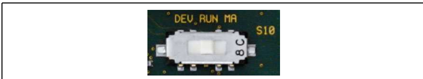
Figure 8.4: DIP switch service - operation
