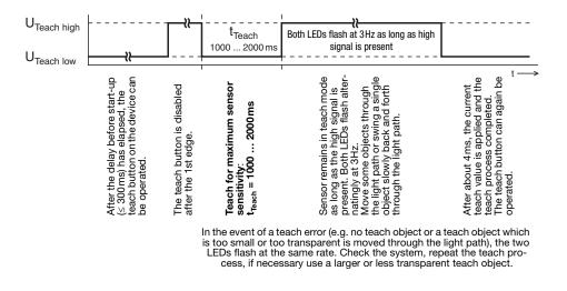
After teaching for maximum sensor sensitivity, the sensor switches for objects with a minimum size of 0.1 ... 0.2 mm (see table under "General Information").
