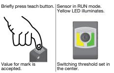
Switching threshold near the mark:
