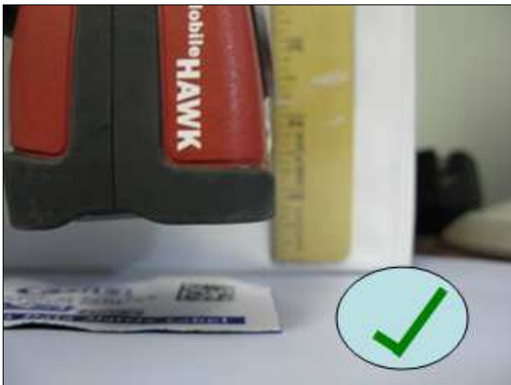
Correct – Move in steadily with front of imager parallel to surface.
