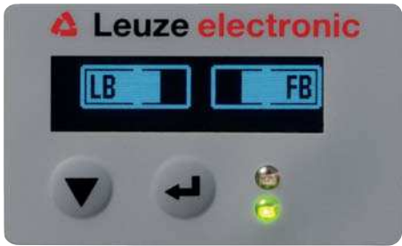
Figure 8.2: Display showing an optimally aligned light curtain
