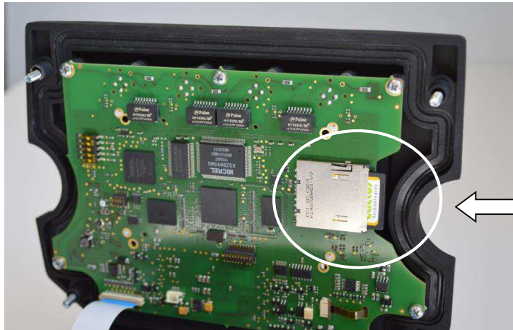
Figure 16 – Removing the Compact Flash
