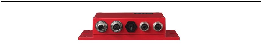
Figure 7.1: Location of the electrical connections
