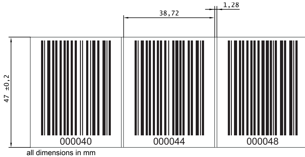
Figure 13.11: Dimensioned drawing bar code tape BCB with 40 mm grid
