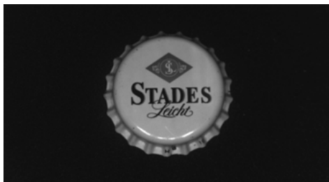
Figure 4.14: Inclined camera alignment with only three illumination quadrants active (reflected quadrant is off) – nearly all reflections in the image are suppressed
