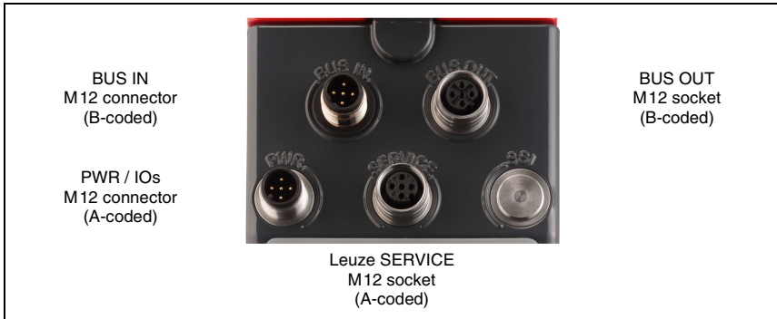
Figure 7.1: Connections of the AMS 384 i
