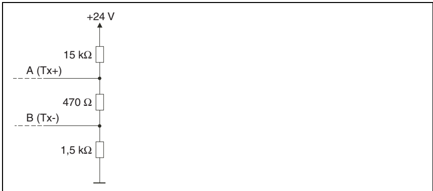
Bild 4.6: Voltage divider for the RS 485 bus termination
