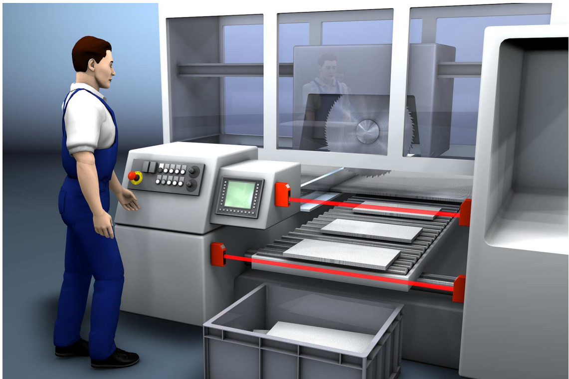
Figure 5.2: Access guarding / intervention control on sawing machines
