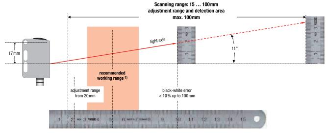
The sensor is most capable of reliably detecting a reflective surface or transparent object in the recommended working range. Nevertheless, the sensor can reliably detect such objects in the entire scanning range; however, the performance reserve is reduced as compared with the recommended working range.
