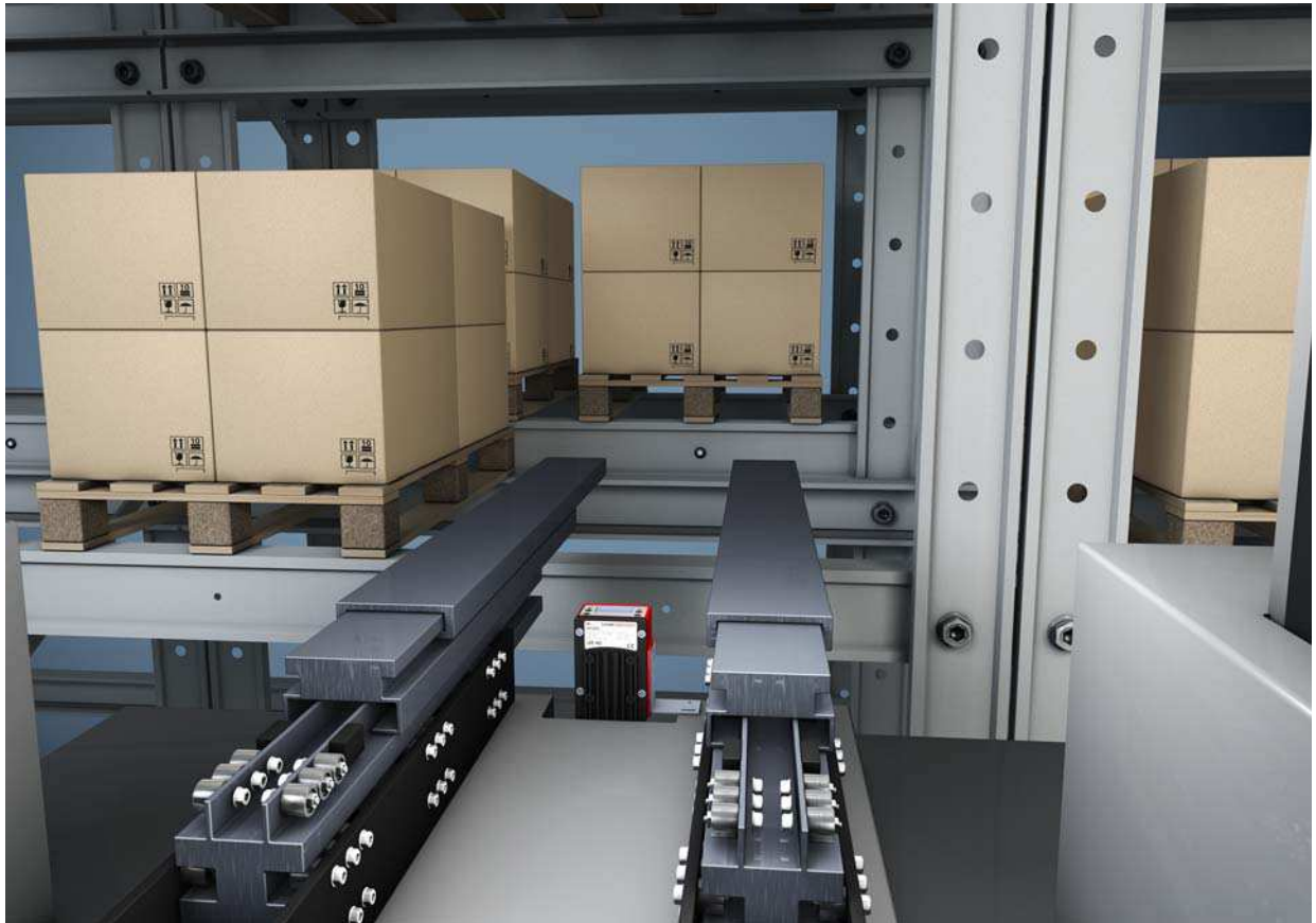
Figure 5.1: Compartment fine positioning of a high-bay storage device in a double-deep pallet high-bay warehouse
