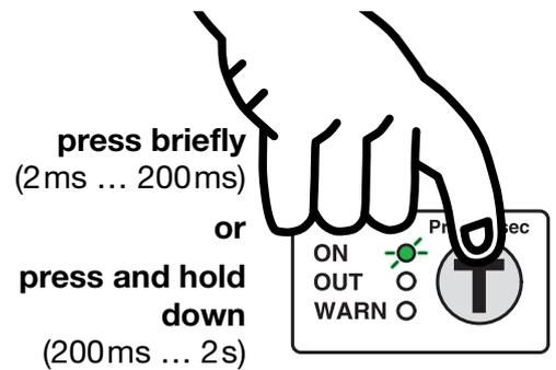
The **green LED flashes one time** quickly or for a longer period time after the button is pressed
