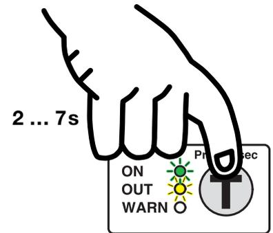
The **green** and the **yellow** LEDs flash **synchronously** approx. 1x per sec.
