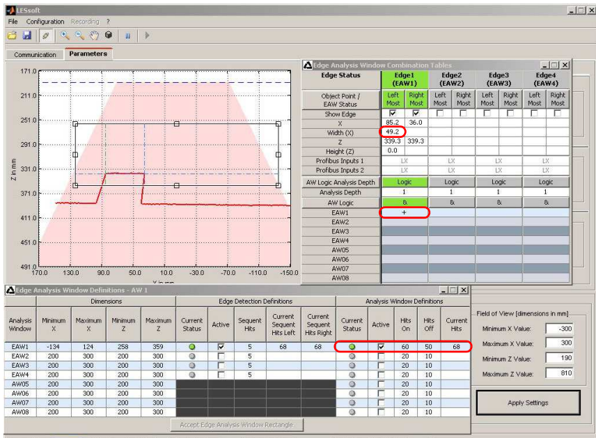
Figure 9.9: Application example 3.1: width monitoring of cubic objects with object detection
