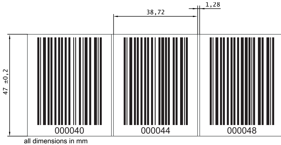
Figure 13.13: Dimensioned drawing bar code tape BCB with 40 mm grid
