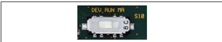
Figure 8.4: DIP switch service - operation
