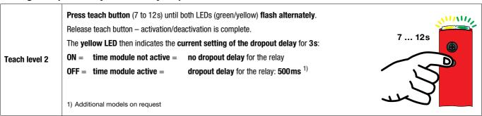
Dropout delay: if the object is no longer present, the output switches with a time delay.
