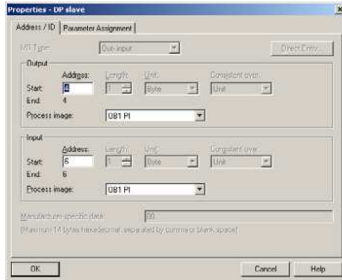
Figure 32: Input/output addresses of the SWD modules in HW config Screenshot of a STEP 7 with courtesy from SIEMENS, Nürnberg
