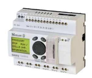
Devices can also be connected to Ethernet, and user-friendly programming with easy Soft CoDeSys provides effective support for creating user programs. It has been optimally designed for electricians and newcomers to automation technology and is the ideal tool for implementing simple applications on easy controllers.
